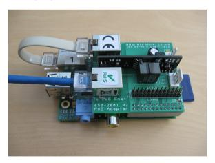
5) Fix the Adapter PCB to the Pi PCB by using the M3 screw (screw the M3 screw into the metal spacer from the underside of the Pi PCB). NOTE: Early Raspberry Pi PCB may not have the fixing holes – in this case see 3) above.
