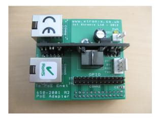
Safety Note: Only use an IEEE 802.3af compatible Switch or Injector with this adapter.
